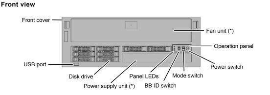
\*: You can see the fan unit and the power unit by removing the front cover.
